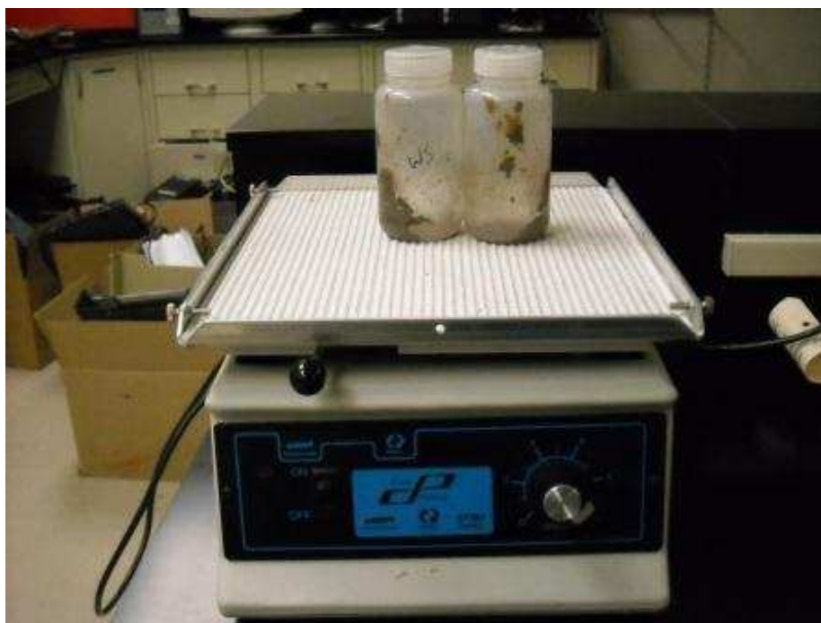
Figure 3.3: Shaker Table and Tubes Used in Fractionation
