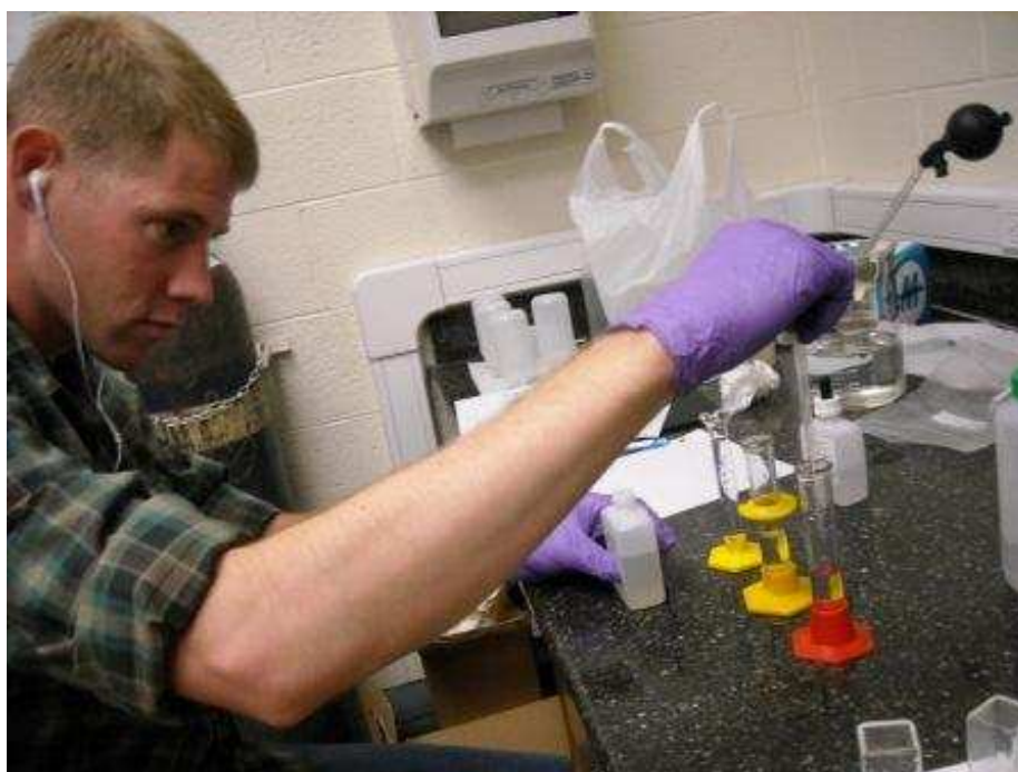
Figure 3.5: Preparing Solutions for Phosphate Measurement Using the Amino Acid Method
