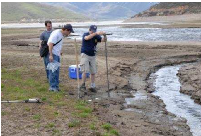
Figure 3.2: Sampling Delta Sediments Using a Hand Auger
