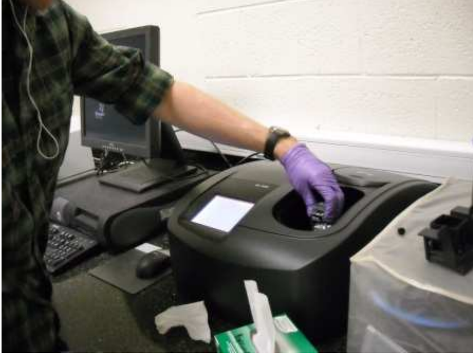
Figure 3.6: Placement of Solution into Spectrophotometer for Measurement
