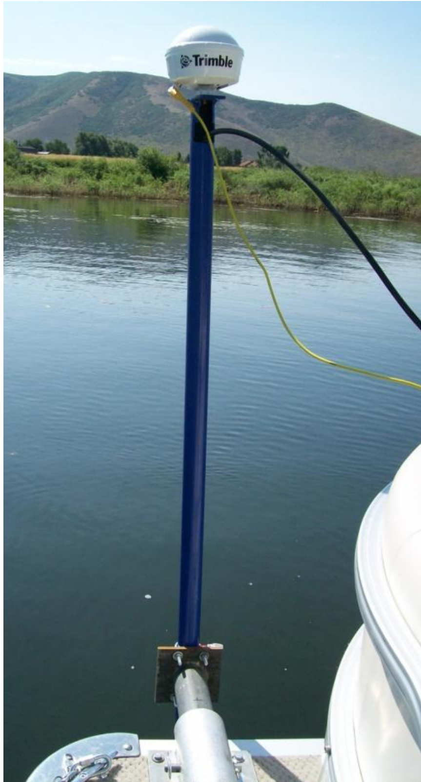
Figure 25: Trimble GPS System and Cable Attached to Sonar
